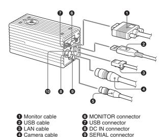
Connect the camera cable to the DC IN connector. Also, if needed, connect the LAN cable to the LAN connector, the monitor cable to the MONITOR connector, the serial cable to the SERIAL connector, and the USB mouse/keyboard to the USB connector respectively.
