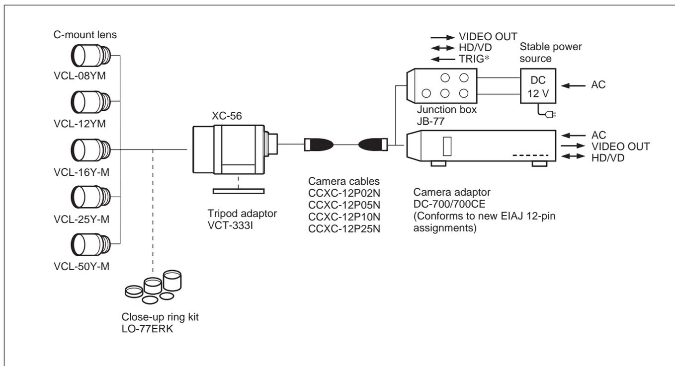
\* If you intend to operate the camera using a trigger pulse, you cannot use the DC-700/700CE. Use the JB-77 Junction Box and a commercially available stable power source, and input a trigger pulse to the CLOCK OUT jack on the JB-77.
