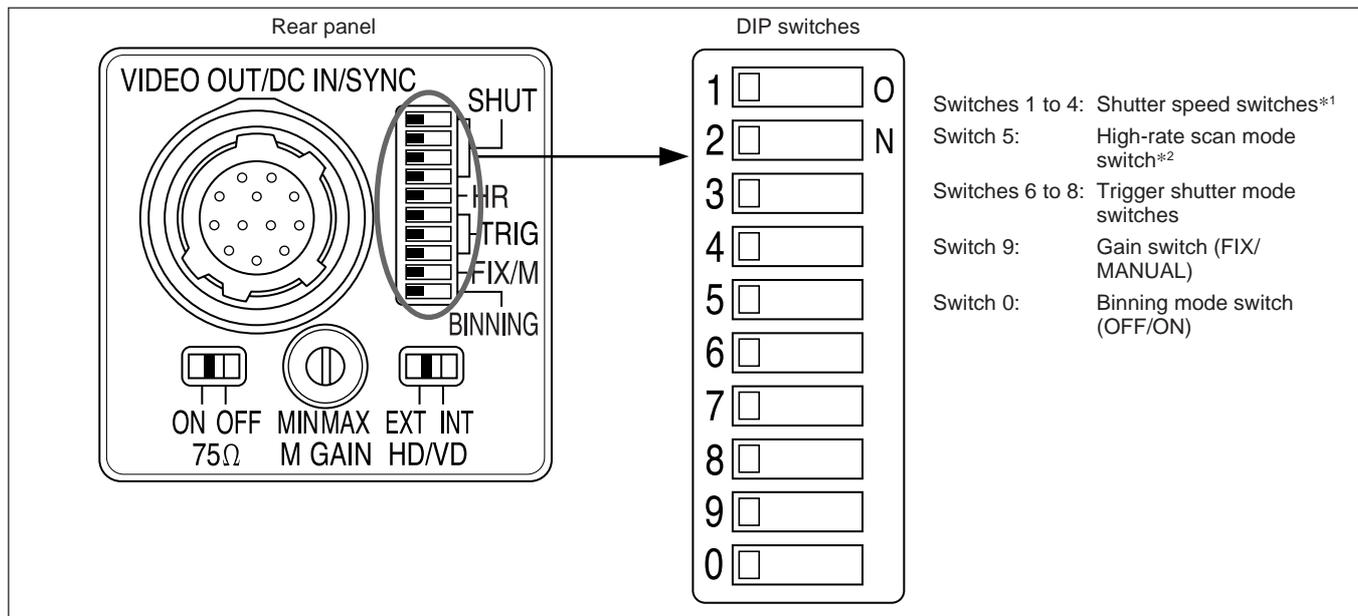
\*<sup>1</sup> The electronic shutter cannot be used in restart/reset mode.
