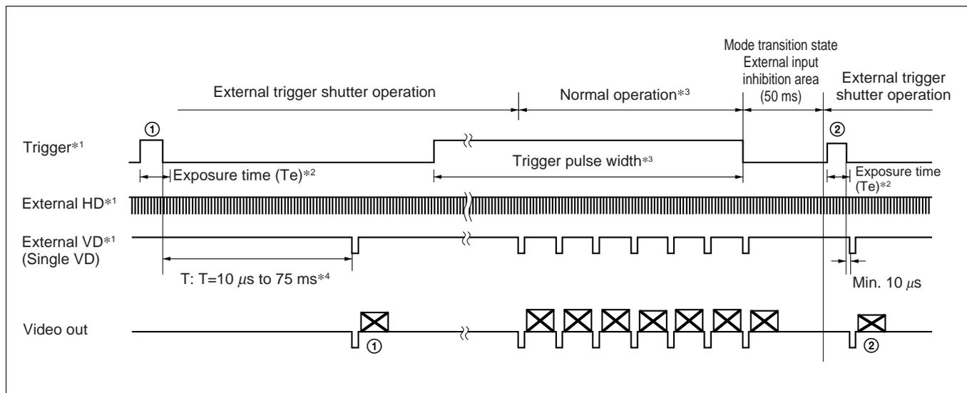
\*1 This is an external input signal. Make sure to input both HD and VD signals in this case. Input the signal so that the VD phase aligns with the HD falling edge.
