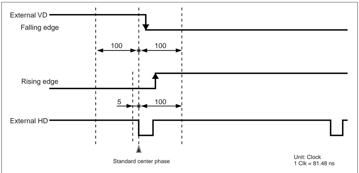
Make sure that the external HD and VD phases against the standard center phase are as shown in the figure.
