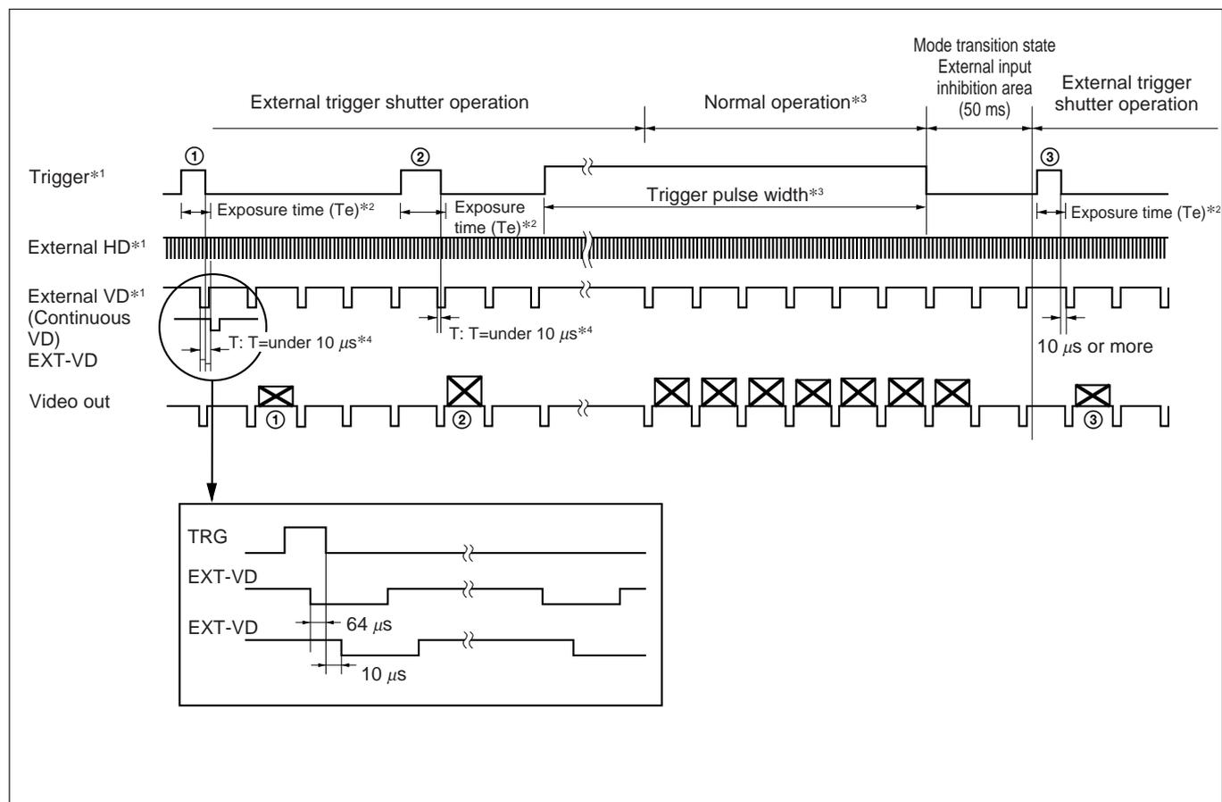
\*1 This is an external input signal. Make sure to input both HD and VD signals.
