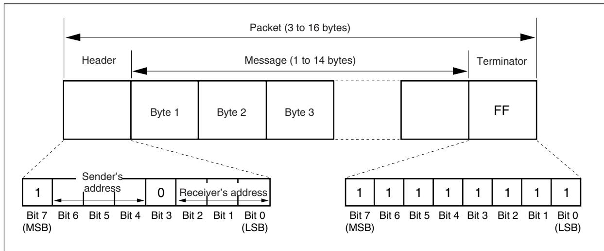
Fig. 2 Packet structure
