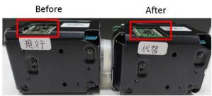
The new circuit board will be located a bit upper side, however it is not over the FCB outside surface.
