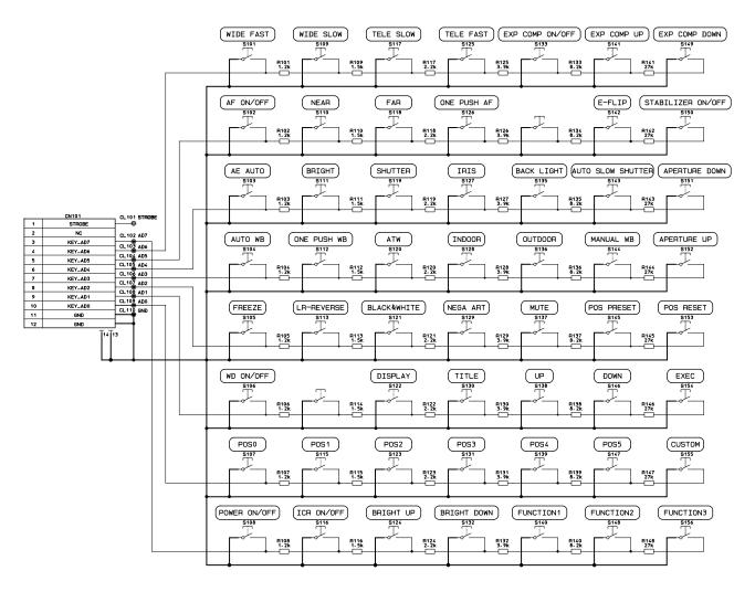
The CN101 is connected to the FCB camera main unit.
