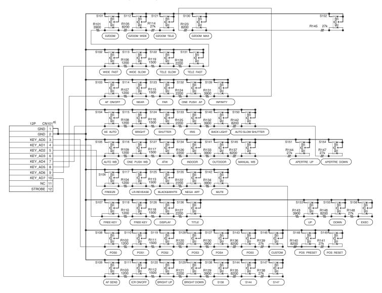
a) The CN101 is connected to the CN601 on the FCB camera main unit.
